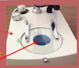
Illuminating specimens from below provides for "transmitted" light viewing and from above for "incident" light viewing. One control switch selects the light source and the other varies ght intensity. To preserve bulb life, IT IS IMPORTANT
