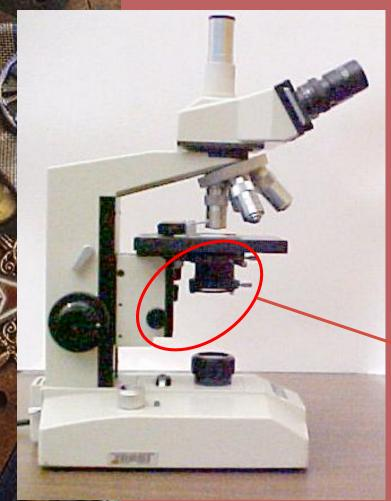
It has its own shutter diaphragm too, for varying the amount of light reaching the specimen slide.
