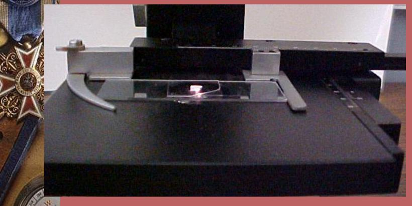
Focusing the microscope on specimen slides can be accomplished with a coarse adjustment control for rapid adjustment, and a fine control for small adjustments, particularly
