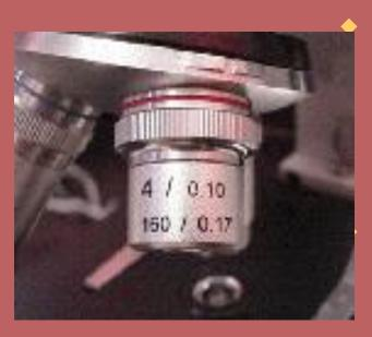
Using the low power objective increases the magnification to 100 times.
