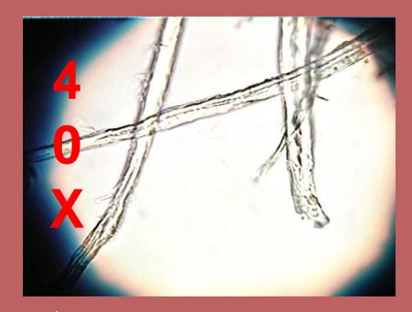
Adjust the condenser diaphragm so that the specimen features are as clearly visible as desired.
