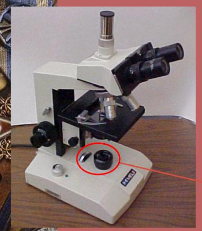
shutter or diaphragm using a control knob to open or close it for more or less light.
