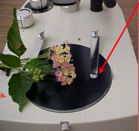
To accommodate large specimens, the entire focusing head of the scope can be raised on the support column. Small specimens can be accommodated by lowering the focusing head on the support column. The illuminator can be moved to provide light as needed for best viewing.
