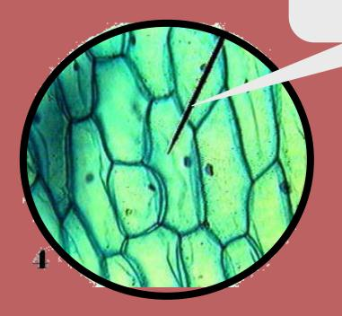
It is a pointer and it moves by turning the eyepiece.
