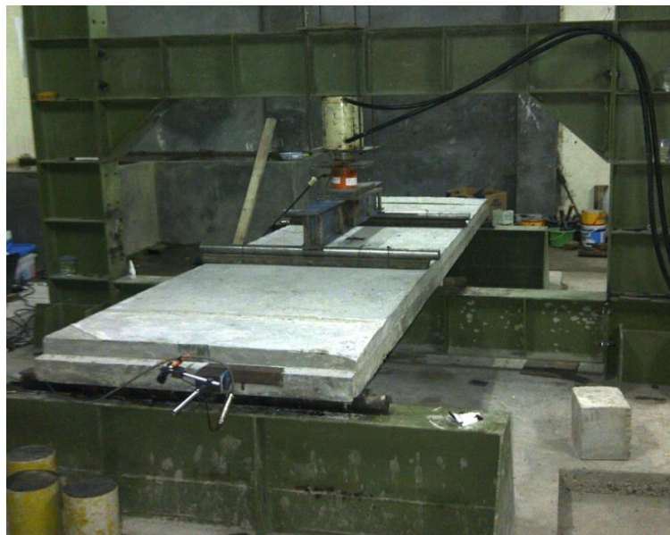
Figure 3 Flexural test setup of the composite concrete slab
