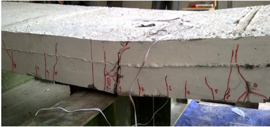
Figure 6. Crack pattern of composite concrete slab that using substrate with as-placed surfaces
