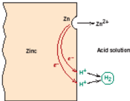
Figure 17.1 The electrochemical reactions associated with the corrosion of zinc in an acid solution. (From M. G. Fontana, Corrosion Engineering , 3rd edition. Copyright © 1986 by McGraw-Hill Book Company. Reproduced with permission.)
