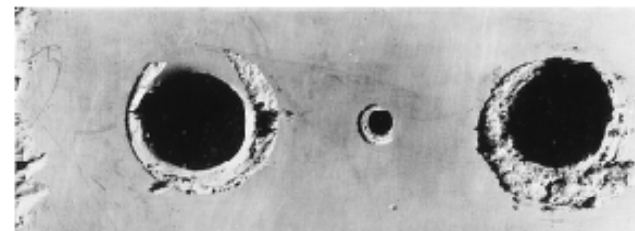
Figure 17.15 On this plate, which was immersed in seawater, crevice corrosion has occurred at the regions that were covered by washers. (Photograph courtesy of LaQue Center for Corrosion Technology, Inc.)
