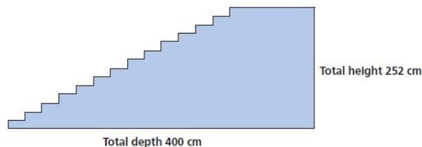
The diagram above illustrates a staircase with 14 steps and a total height of 252 cm:
