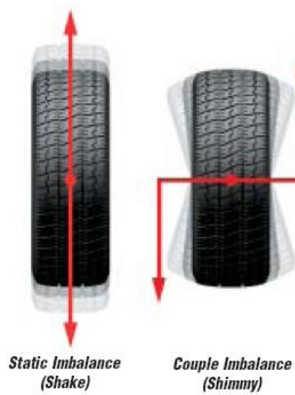
Gambar 62. Ilustrasi tipe unbalance roda
