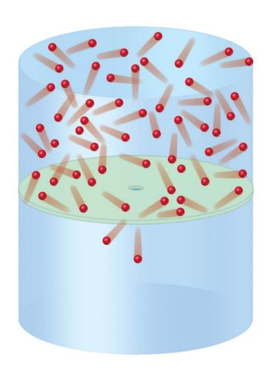
The escape of gas molecules through a tiny hole into an evacuated space.
