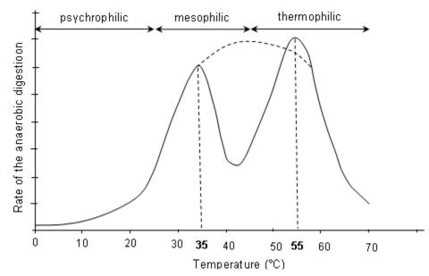
**Figure 2.2** Influence of temperature on the rate of anaerobic digestion process. Optimum temperature for mesophilic around 30 - 40 °C and for thermophilic 50 - 60 °C
