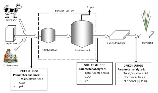
Figure 3.2 Sequence and sampling procedure for multi substrate digestion
