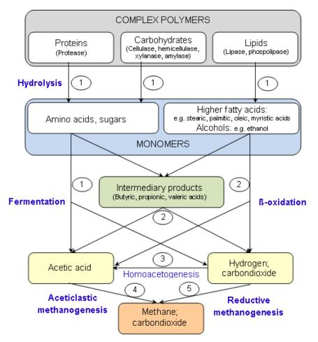
**Figure 2.1** Schematic diagram of complete anaerobic digestion of complex polymers. Names in brackets indicate the enzymes excreted by hydrolytic bacteria. Numbers indicate the bacterial groups involved:
