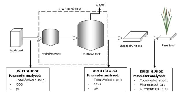
Figure 3.1 Sequence and sampling procedure for sole substrate digestion
