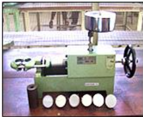
Gambar 5.17. Universal strength machine tipe PFG
