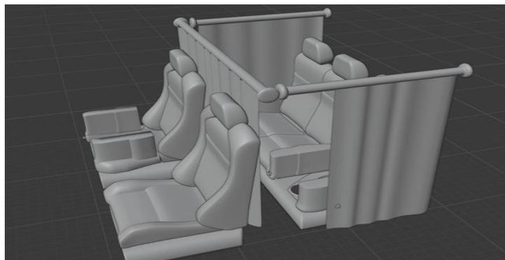
Figure 6. Car seat emergency toilet design complet
