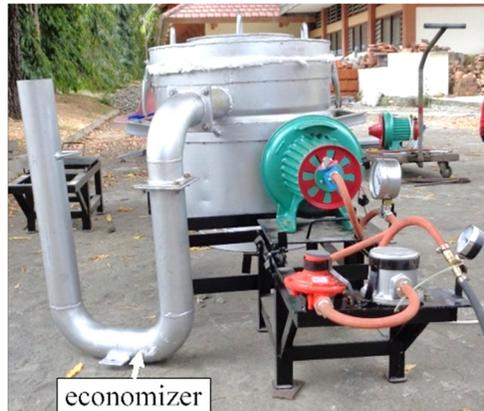
FIGURE 1. Crucible furnace with economizer [5]
